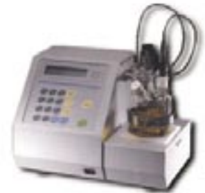
Portable Karl Fischer Titrator CA-21 Validation of data by Primary Standard in the Field
