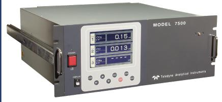
A high-sensitivity mass flow sensor is utilized for infrared measurements. By using a single beam, single path design in conjunction with a serial dual-layer transmission detector, the 7500 delivers long-term, drift-free performance. The oxygen concentration in the sample gas can be detected by either a built-in paramagnetic sensor, Micro-fuel cell, or an externally mounted, in-situ-based zirconium oxide sensor.
