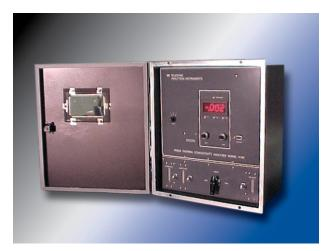
Designed to detect a specific impurity in a binary gas mixture, the 212R is also well suited for monitoring one component in more complex mixtures where the other gases have the same ratio to each other or have similar thermal conductivity coefficients.
